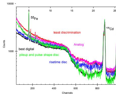
Figure 3. Manganese and silver K x-rays spectra superimposed on  $^{133}\text{Ba}$  nuclear and Compton background. The shape of the Compton profile depends on the signal processing approach.
