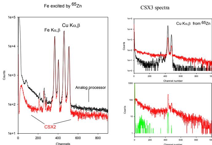
Figure 1. An Fe sample is irradiated with Cu K radiation from a  $^{65}\text{Zn}$  source in transmission geometry. The background is substantially reduced using the CSX2 or CSX3 by noise discrimination and risetime discrimination. The manufacturers analog processor (—), and the Cambridge Scientific CSX2 digital processor (—).
